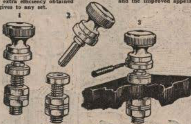
1. Complete Terminal—actual size. 2. Terminal disassembled. 3. Terminal with wire joined—mounted on panel.
